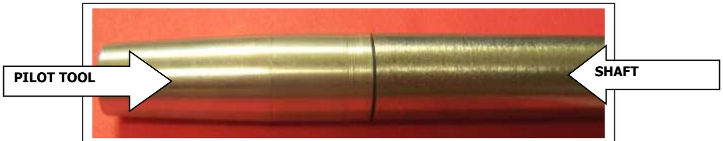
7. Remove the Harley shaft a little at a time while simultaneously from the opposite side start inserting the Mad Dog shaft from the pilot tool side.
