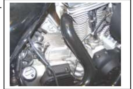
4. Support the trans to relieve pressure on rear fork (swing arm) and remove any footboards and brackets, rubber mounts, and hardware.
